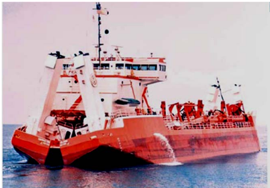
Figure 5-2. Split-Hull Hopper Dredge Manhattan Island Bottom Dumping Material (Source: Great Lakes)
