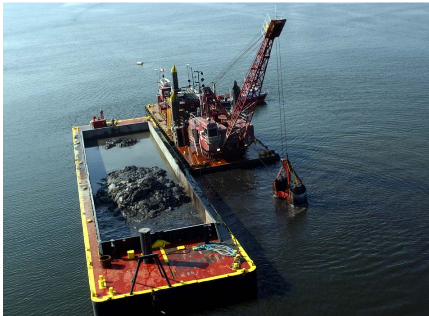
Figure 5-1. Clamshell Dredge and Scow (Source: Great Lakes)
